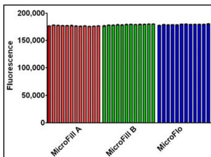
**Figure 5. Dispense Uniformity of Reagent Dispensers.** The different dispenser modules were used to dispense 5  $\mu$ L of lysis buffer containing fluorescein dye into 192 wells of a 384-well microplate. The fluorescence was determined using a Synergy 2 Multi-Mode Microplate Reader. Each data points represent the mean of 16 wells.
