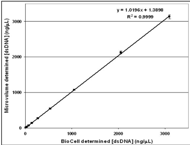
**Figure 4.** Accuracy of micro-volume quantification of dsDNA relative to measurements made at 1 cm path length with BioCell™ accessory. Both micro-volume and BioCell measurements are made with the Take3™ Multi-Volume Plate.
