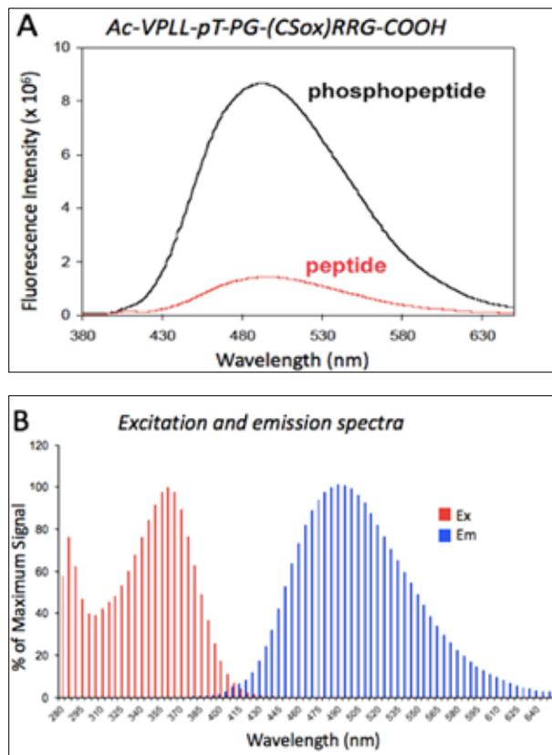
**Figure 2. Fluorescence Spectra of PhosphoSens<sup>®</sup> Peptides.** (A) Typical fluorescence changes upon phosphorylation of a peptide substrate for ERK1/2 MAPK: Ac-VPLL-pT-PG-[CSox]-RRG-COOH. (B) Excitation and Emission spectra. The  $\lambda_{ExMax}$  of chelated Mg(II) with the 8-hydroxyquinoline is 360 nm and the  $\lambda_{EmMax}$  is 485 nm.
