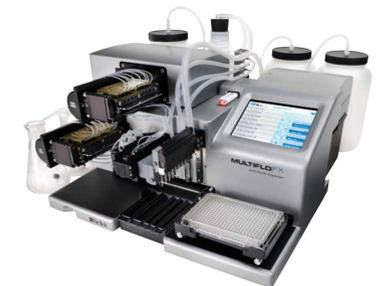
**Figure 14. MultiFlo FX Multi-Mode Dispenser.** The MultiFlo FX is a modular upgradable reagent dispenser that can have as many as two peri-pump (8 tube dispensers), two syringe pump dispensers and a strip washer. The syringe and washer manifolds can be configured for plate densities from 6- to 384-well.
