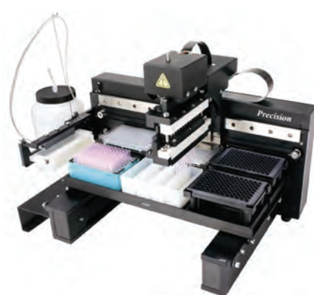
Figure 2 – The Precision™ Microplate Pipetting System combines an 8-channel pipetting head and an 8-channel bulk reagent dispenser in one instrument. The instrument was used to dispense all assay components, including target and effector cells, serially titrate antibody across a 96-well PP plate, transfer samples from plate to plate, as well as dispense the aCellaTOX assay components.
