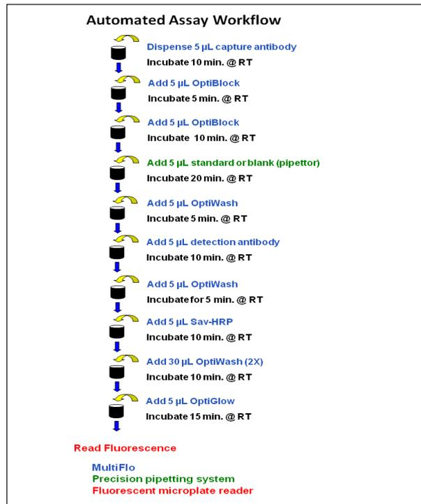
Figure 2. Automated Workflow.
