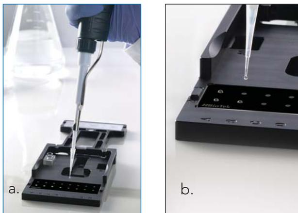
**Figure 1.** Take3 Multi-Volume Plate shown with BioCell™ in place (a). Two additional locations are available for a second BioCell and a standard cuvette. Sample volumes as low as 2  $\mu$ L can be loaded on 16 microspot locations using either a single- or multi-channel pipettor.
