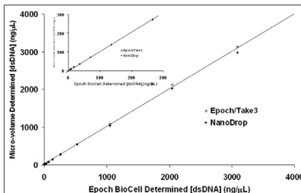
**Figure 3.** dsDNA standard curve using dilutions of a purified herring sperm sample. Abscissa data is considered actual [dsDNA] as measurements were conducted with 1 cm pathlength using BioCell™. Ordinate data is micro-volume determinations using Epoch™ Spectrophotometer System and NanoDrop. The straight line is through the origin and has a slope of 1.000, which is considered a perfect equivalence between micro-volume and BioCell data. Inset is an exploded view of low dsDNA concentrations.
