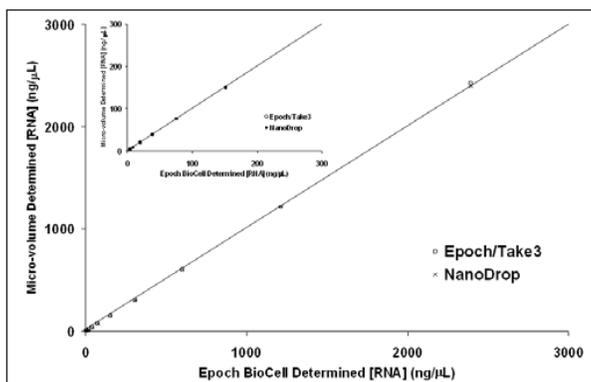
**Figure 4.** RNA standard curve using dilutions of a purified yeast RNA sample. Abscissa data is considered actual [RNA] as measurements were conducted with 1 cm pathlength using BioCell. Ordinate data is micro-volume determinations using Epoch Spectrophotometer System and NanoDrop. The straight line is through the origin and has a slope of 1.000, which is considered a perfect equivalence between micro-volume and BioCell data. Inset is an exploded view of low RNA concentrations.
