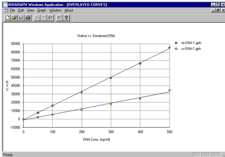
**Figure 3. Comparison of OliGreen™ fluorescence with native and denatured DNA.** Concentration curve from 0 to 500 ng/ml of either heat denatured or native purified salmon sperm DNA with linear regression analysis. Data indicated were recorded with a sensitivity setting of 120 and has been corrected by subtraction of a 0 ng/ml blank.
