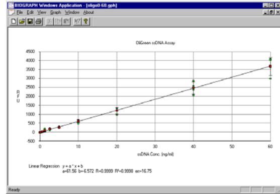
**Figure 1. Concentration curve of pUC forward primer oligonucleotide.** (A) Concentration curve from 0.0 to 900 ng/ml of pUC forward primer oligonucleotide with linear regression analysis. (B) Concentration curve from 0.0 to 60ng/ml of pUC forward primer oligonucleotide with linear regression analysis. Data indicated were recorded with a sensitivity setting of 125 and has been corrected by subtraction of a 0 ng/ml blank.
