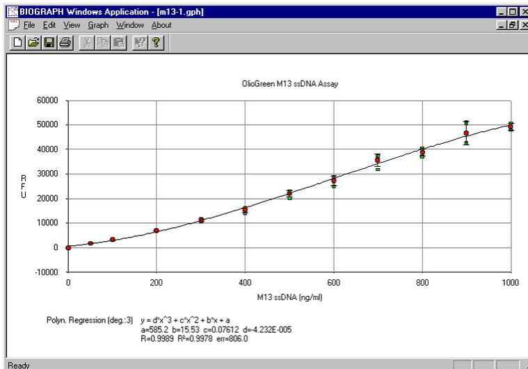
**Figure 4. Concentration Curve of M13mp18+ viral DNA.** Concentration curve of M13mp18+ ssDNA from 0 to 1000 ng/ml with polynomial curve fit of the data. Data indicated were recorded with a sensitivity of 120 and has been corrected by subtraction of a 0 ng/ml blank.
