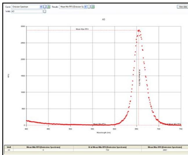
**Figure 2. Emission Scan of Qdot 655 nanocrystals.** Using an excitation wavelength of 340 nm, the emission from 400 nm to 750 nm spectra in 1 nm increments was obtained using a Synergy 4 Multi-Detection Microplate Reader.
