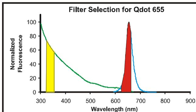
**Figure 6. Filter Selection Based on Fluorescent Scans.** Fluorescent excitation (—) and emission (—) scans from Qdot 655 were performed using a Synergy 4. The bandpass of the selected excitation (■) and emission (■) filters were then superimposed on the plots.
