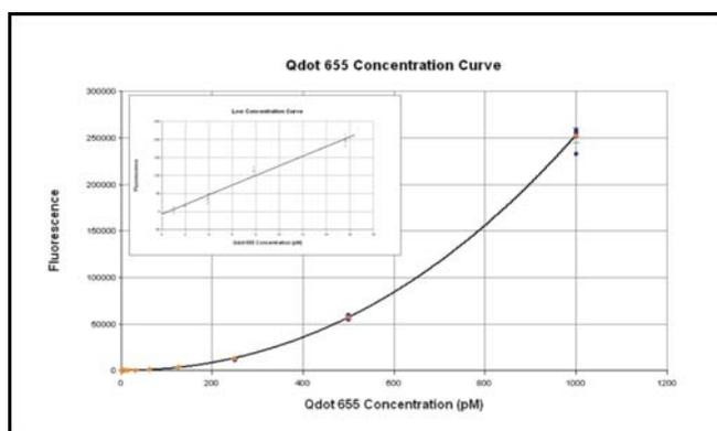
**Figure 7. Qdot 655 Concentration Curve.** The fluorescence of a series of dilutions ranging from 0 to 1000 pM of Qdot 655 was determined using a Synergy 4 reader with a 340/40 excitation and a 645/40 emission-filter. The reader was controlled and the data collected and plotted using Gen5™ Data Analysis Software (BioTek Instruments).
