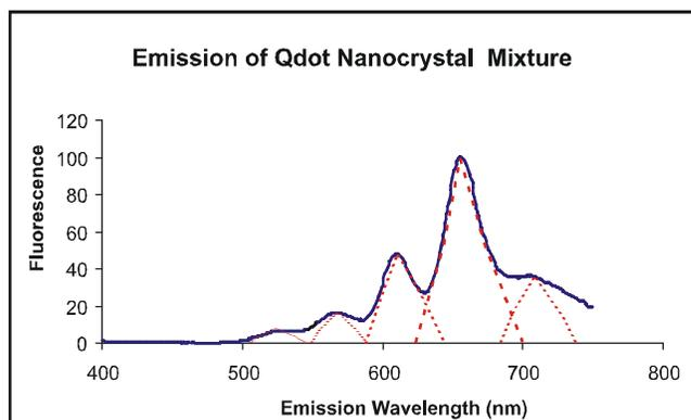
**Figure 5. Fluorescence emission scan of a Qdot mixture.** Equimolar (1 nM) amounts of Qdot 525, 565, 605, 655, and 705 were excited at 340 nm and the fluorescent emission measured from 400 nm to 750 nm in 1 nm increments. Solid blue line indicates the actual fluorescence, while dashed red lines indicate estimated signal of each Qdot nanocrystal.
